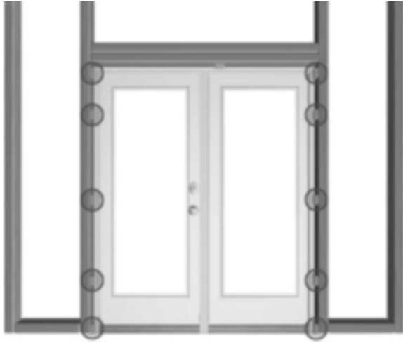
Figure 16: Install the shims in the correct locations and in the correct sequence.
