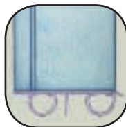
Triple Contact Bottom Sweep Twin compression bulbs and an extruded vinyl "blade" mate with the adjustable threshold to seal the door bottom. Helps eliminate drafts, leaks and ice build-up.
